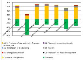
The phases of extracting raw materials and repairs have a dominant influence on all environmental impacts. In particular, the drive unit installed in the product and the high mass percentages of glass and aluminium processed in the sliding panels and side screens are responsible for this. On the other hand, energy use during manufacturing is only of subordinate significance as it is provided in full by hydropower.
